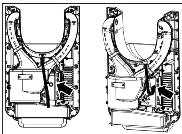
Assembly the supplied hose to the hand dryer back. Assembly the the hand dryer to the wall, placind the assembled hose inside the wall drain pipe.
